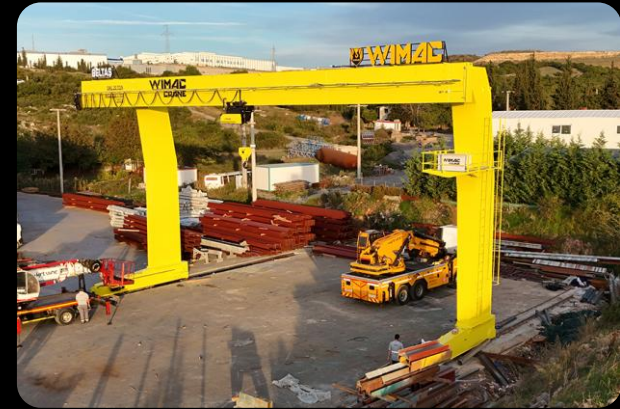
L-Type Single Girder Gantry Crane (SWL 20 MT)
